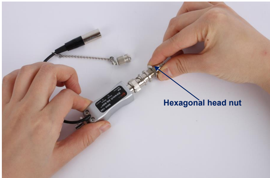
Fig. 3: Connection of the BNC bulkhead receptacle into BNC connector of SDIX-100
