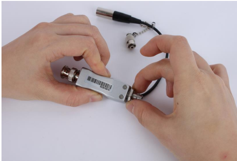
Fig. 1: Screwing smaller hexagonal head nut at ST connector side
