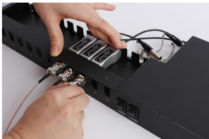
Fig. 7: Connection of BNC cables into the BNC receptacle of SDIX-100
