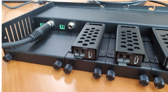
Fig. 6: Mounting the Module bracket on BR-500.
