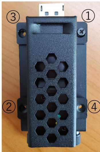
Fig. 4: Holes to insert the screws
