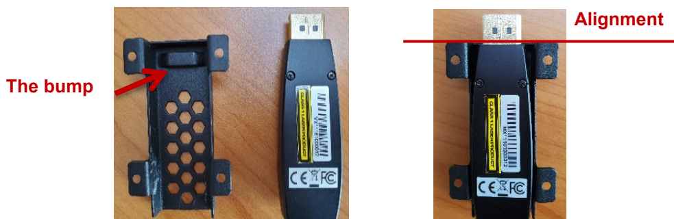
Fig. 2: Insert the push button into the bracket
