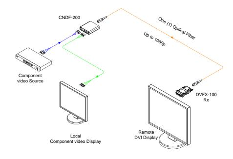
Figure 1 - Connection Diagram of CNDF-200
