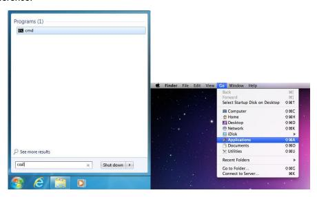
Once in the CLI (Command Line Interface) type "telnet" followed by the IP address of the unit (and the port number if it is non-standard) and then press "Enter"
