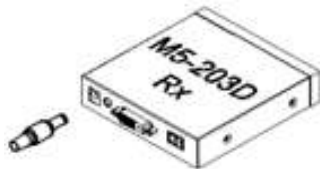
Figure 3 – Connection of power adapter to the receiver
