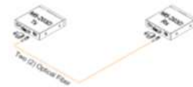
Figure 4 – Connection of optical fibers
