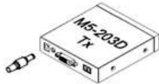
Figure 2 – Connection of power adapter to the transmitter
